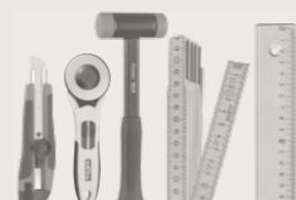
Necessary tools for laying: cutter (straight blade and curved blade), rubber mallet, measuring tape, ruler - set square.
